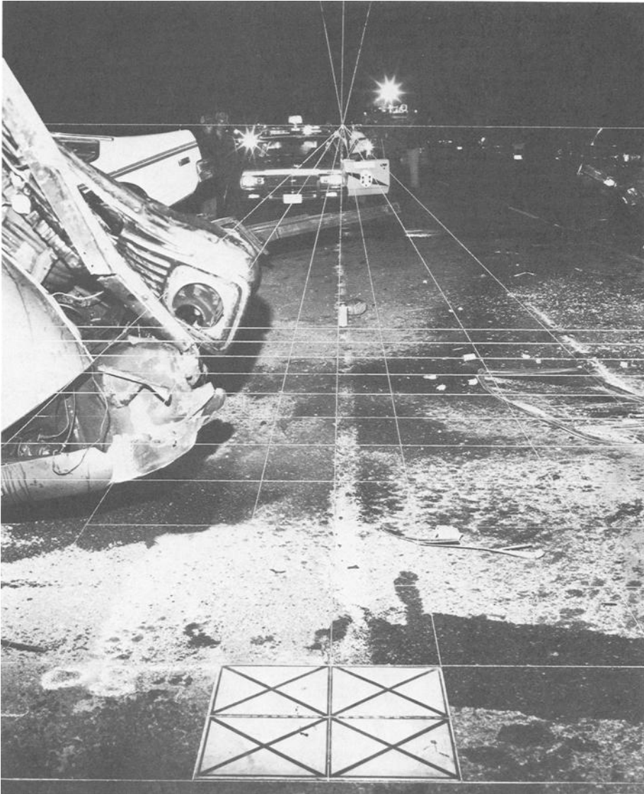
FIG. 1—Perspective grid technique applied to automobile accident scene measurements. (Photo courtesy of Jack Whitnall.)
